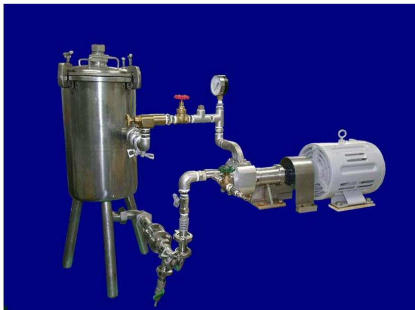
**Fig. 4 Pressurizing centrifugal pump**
